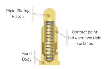
A rigid contact point will disconnect under shock and vibration conditions. This solution is only suitable in static-mode and low current applications. Spring Loaded Contacts
