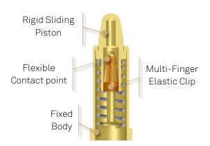
An integrated Multi-Finger elastic clip establishes a reliable and efficient multi point connection between body and piston. Flexible contact is compliant to shock and vibration up to 2000Hz or more, and capable to handle currents up to 20A.
